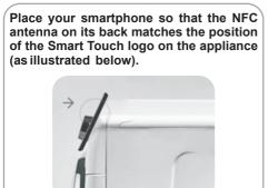
If you do not know the position of your NFC antenna, slightly move the smartphone in a circular motion over the Smart Touch logo until the App confirms the connection. In order for the data transfer to be successful. it is essential TO KEEP THE SMARTPHONE ON THE DASHBOARD DURING THESE FEW SECONDS OF THE PROCEDURE; a message on the device will inform about the correct outcome of the operation and advise you when it is possible to move the smartphone away.
